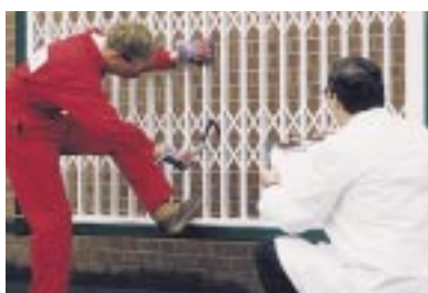
SecuroGuard 1001 undergoing a simulated attack test
